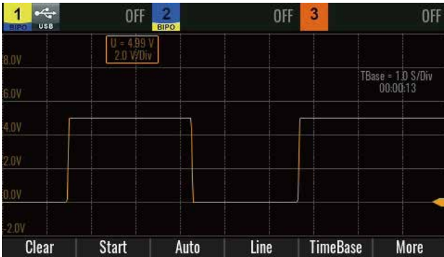
Trend Chart Analysis for Monitoring Long-Term Voltage, Current, and Power Curves of DUT, with Real-Time Data Saving to USB Drive
