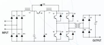
Simplified topology diagram for Magna-Power's current-fed power processing
