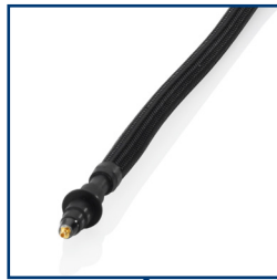
R&S®ZISO-Z101/-Z201 MMCX probe tip
