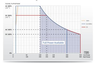
All Asterion sources employ AMETEK's latest current enhancing technology, iX2™. iX2 current doubling technology enables output current to increase linearly up to two times the full voltage current as the voltage decreases from range maximum to one-half of range voltage. iX2 technology results in a source that **DELIVERS FULL POWER OVER THE WIDEST VOLTAGE RANGES!** This eliminates the need to buy overpowered sources just to reach low line current requirements.
