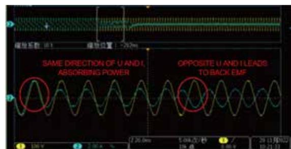
IT7900P simulates the motor from loading to generating back EMF
